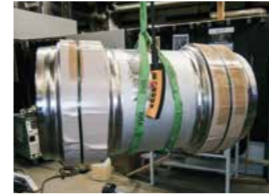
Cleaned with osmotic water, the expansion joint is now ready for dispatch.
