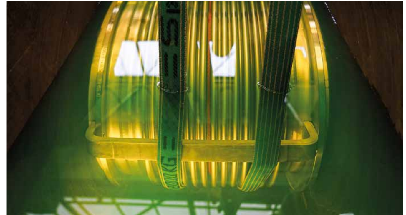
Pressure and leakproof testing in special liquid bath.
