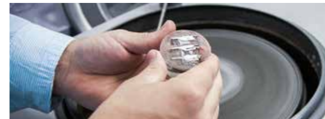
Under the scanning electron microscope, microsections of different materials (Mu-metal, magnifer and 1.4571) provide information about their changed microstructure after processing.
